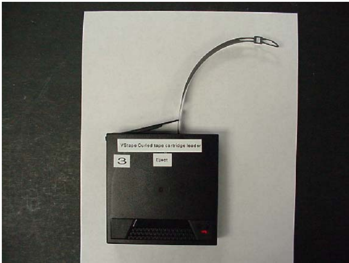
Tape leader is curled such that it is no longer in the correct position.
