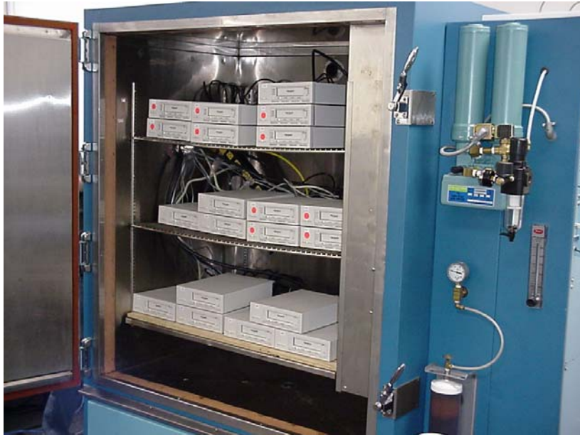
Figure 5: Temperature & Humidity test set up
