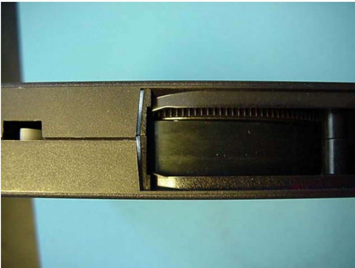
Tape cartridge is missing the tape cartridge leader.
