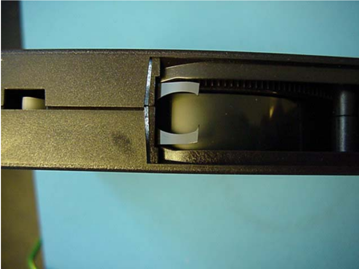
Tape has the tip of the buckle broken off.
