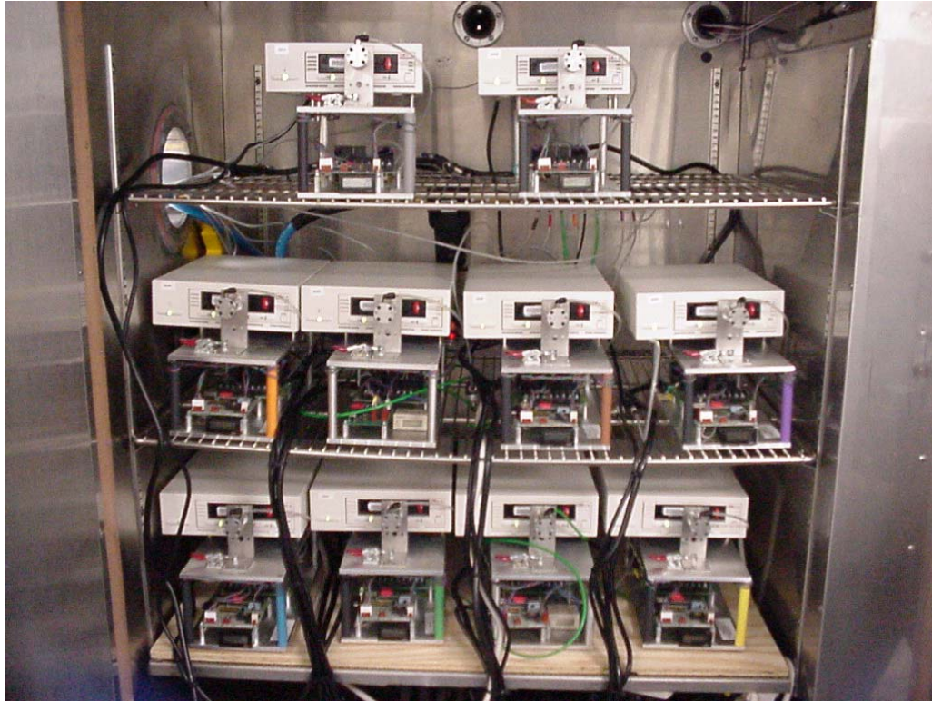
Figure 6: VS160 Drives on Load/Unload Fixtures in Thermal Chamber
