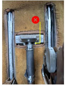
• Extending (Gear Down): The gear handle must be Fully seated in the holder, and locked, and green indicator
